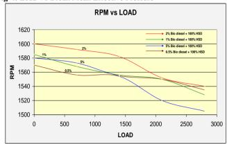
Fig.-5: RPM Vs Load
