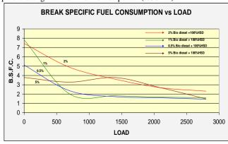
Fig.2: Load Vs Fuel Consumption
